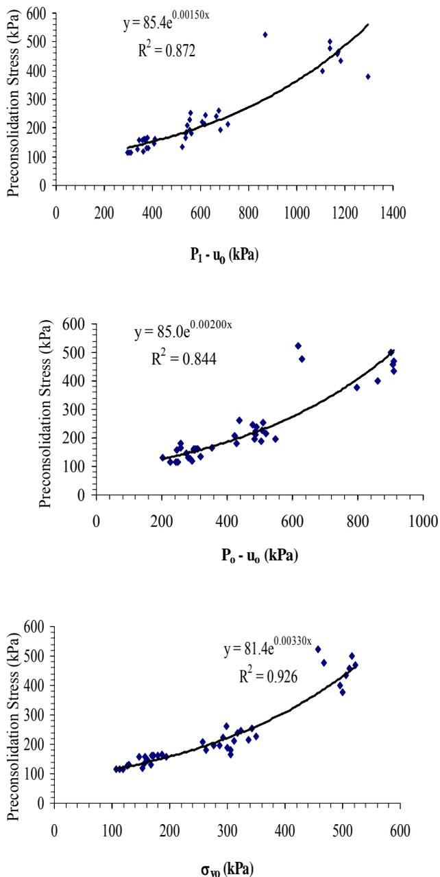
Figure 2. DMT Correlations, Dilatometer  $(P_1 - u_o)$  vs. Laboratory Determined  $\sigma'_p$ , Dilatometer  $(P_o - u_o)$  vs. Laboratory Determined  $\sigma'_p$ , and Total overburden stress,  $\sigma_v$  vs.  $\sigma'_p$
