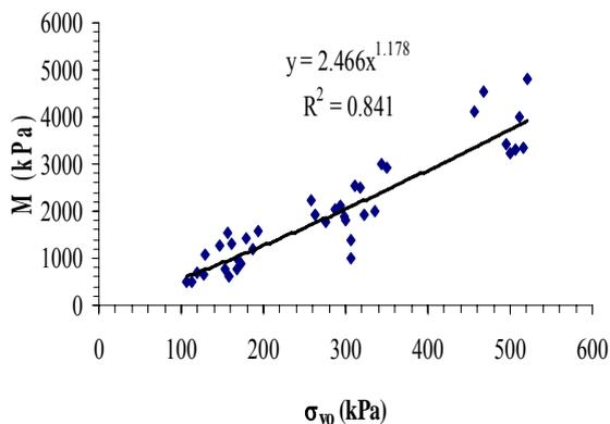
Figure 6. DMT Correlations, Dilatometer  $(P_0 - u_o)$  vs. Laboratory Determined  $M$ , Dilatometer  $(P_1 - u_o)$  vs. Laboratory Determined  $M$ , and Total Overburden Stress vs.  $M$
